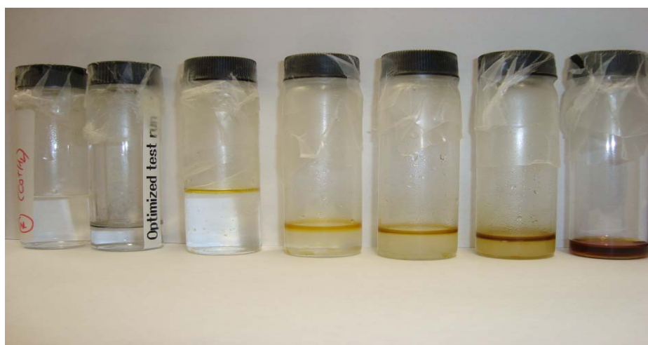
Fig 3. Fuel samples 1-7 showing the change in phase separation as the optimal 2:1 H 2 :CO ratio is reached. Sample #7 is the resulting optimized fuel as seen in the GC results of Fig 1.
