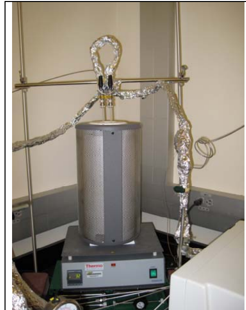
Figure 2. Here is a closer look at the heated region of the micro-reactor. The heater is raised into place to control the temperature of the quartz u-tube while a gas mix is flowed through reactor.
